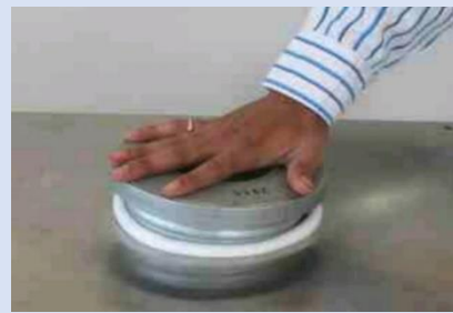
Press the Cartridge Filter into the snap cuff
