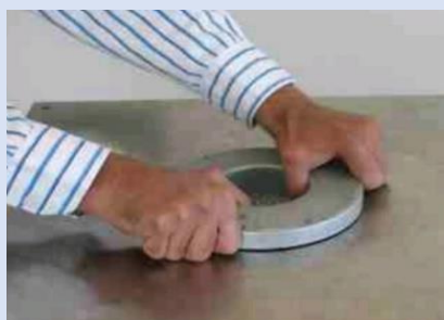
Pull the Cartridge Filter with Hands step by step
